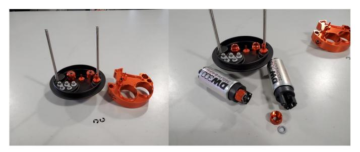
2 – Install the supplied longer 6" x 5/16" convoluted tube onto the return fitting and secure with the supplied 5/16" pinch clamp. Slide the center plate over the pumps and return tube, reinstall the e-clips, cut the return hose flush with the bottom of the return plate when its fully extended.
