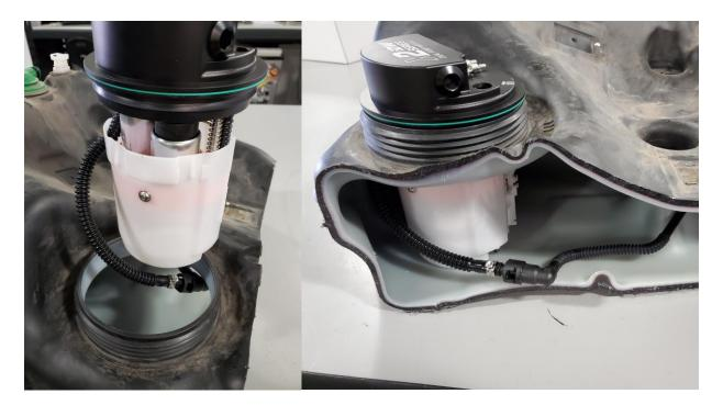
16 – There are no physical alignment tabs or notches on the GT86 module and fuel tank. Instead, there is an alignment marking on the DW X2 module and a corresponding marking on the OEM fuel tank.
