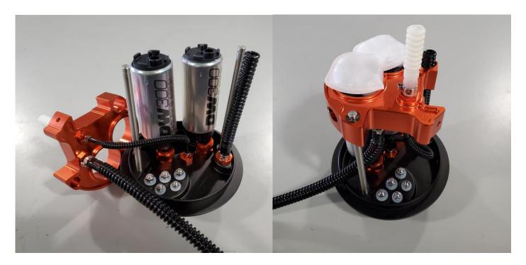
6 – Shorten the supplied wiring harness to approx. 8-inch (205mm) and crimp on the supplied 14-16awg ring terminals. Attach both ground wires to the pump negative terminal and attach each pump power wire to its separate positive terminal. Tuck the remaining wire into the cavity provided above the pumps.
